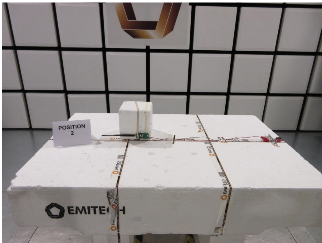
TEST SETUP PHOTO(S) - BAND-EDGE / POSITION 2
