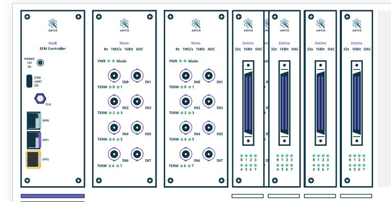
i It is recommended to use 2 EEM connectors for Novo, but it is possible to use only 1 EEM connector.
