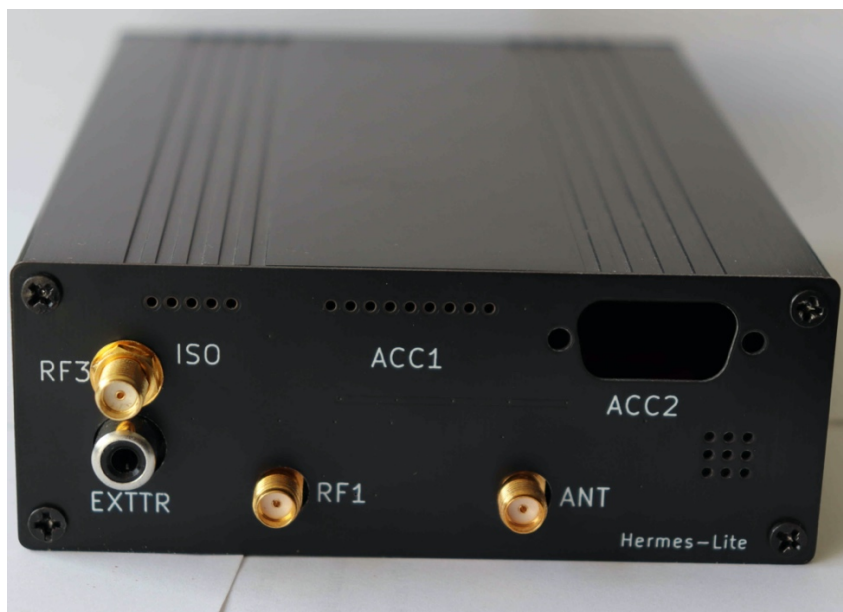
Fig. 8. Back view of the HL2 case, showing the new RF3 jack near the top left corner
