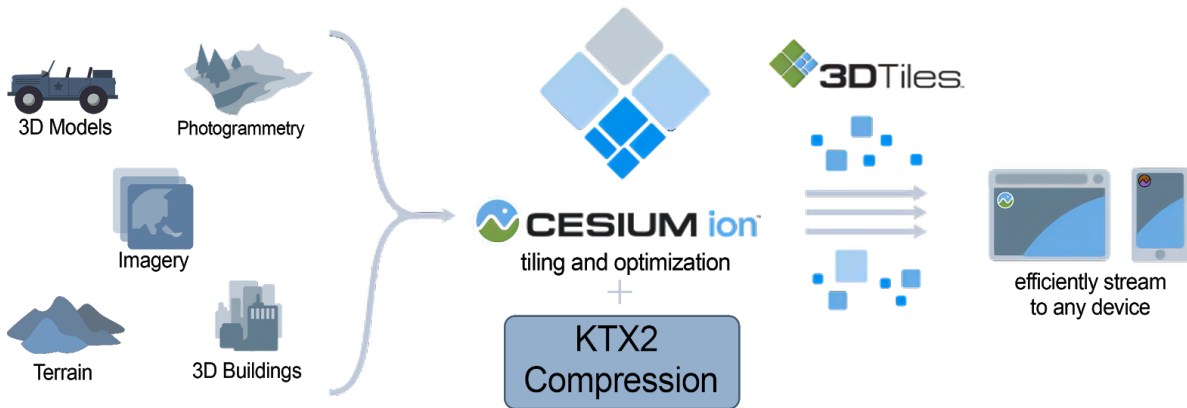
Figure 3. A representation of the pipeline used to create and evaluate KTX2 for storage and streaming into CesiumJS that was used to evaluate the results for this report.
