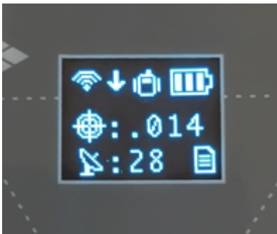
Rover with Active NTRIP Client Connection
