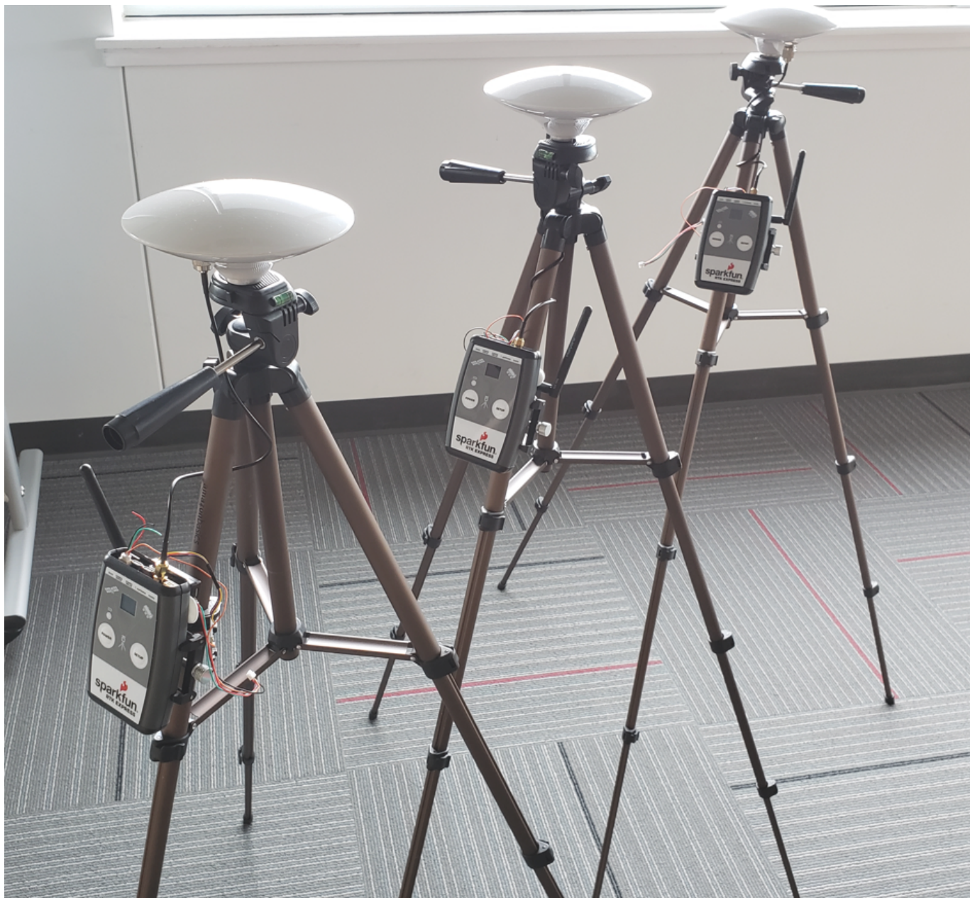
Three RTK Expresses wired with external microphones
