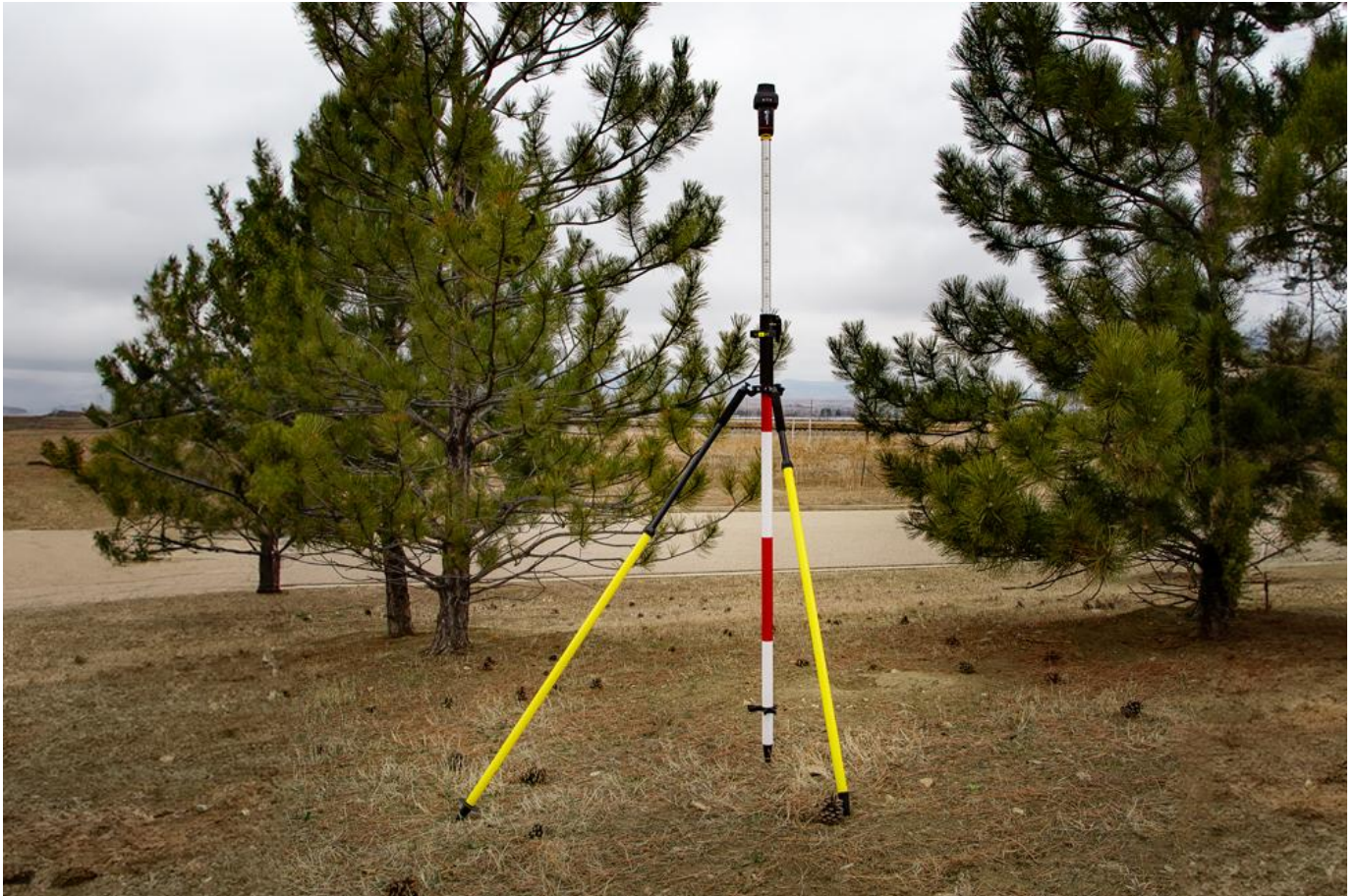
RTK Torch on a Monopod + Bipod
