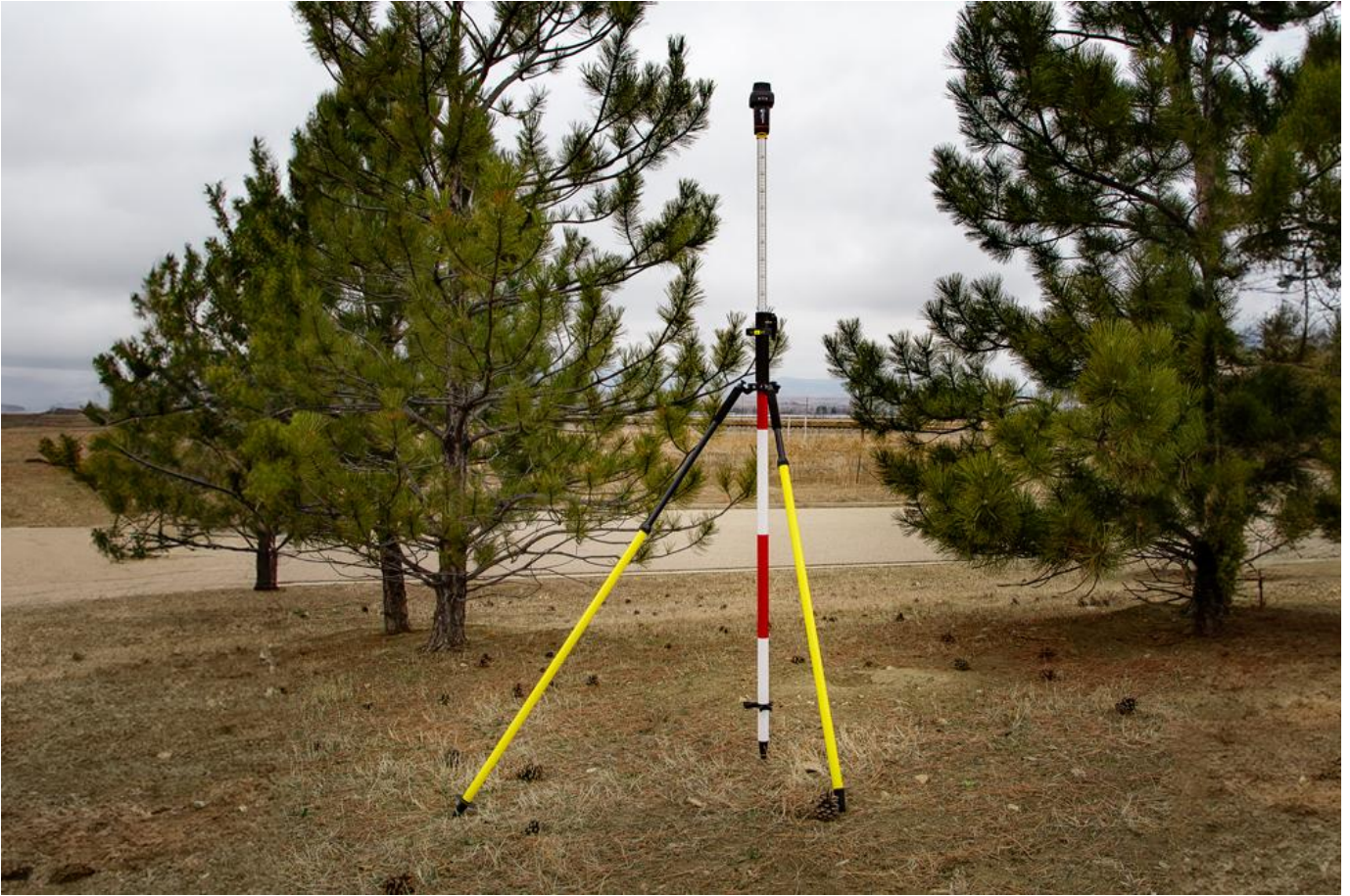
RTK Torch on a Prism Pole with Bipod
