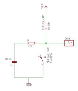
NO (normally open) switch (PROBE) connected to D18 (Zmin) with pull-up resistor. R and C form a low-pass R-C filter needed to filter noise.
