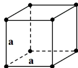
$$\begin{aligned} \therefore E(\vec{k}) &= \varepsilon_s - J_0 - J_1 \left( e^{ik_x a} + e^{-ik_x a} + e^{ik_y a} + e^{-ik_y a} + e^{ik_z a} + e^{-ik_z a} \right) \\ &= \varepsilon_s - J_0 - 2J_1 \left( \cos k_x a + \cos k_y a + \cos k_z a \right) \end{aligned}$$
