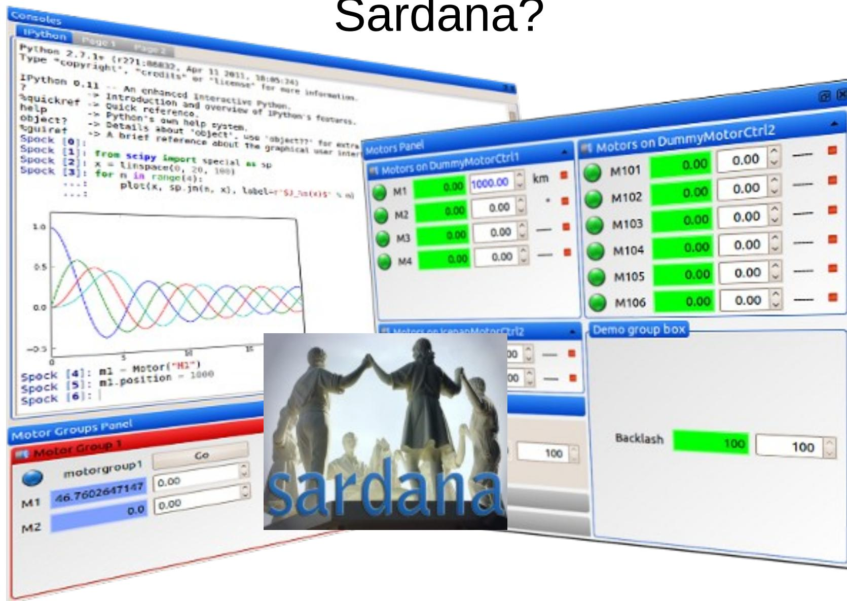
**Sardana** is a SCADA for scientific installations originally developed at ALBA.
