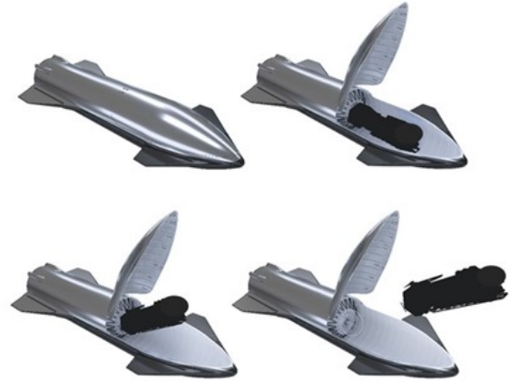
Figure 3: Starship payload deployment sequence
