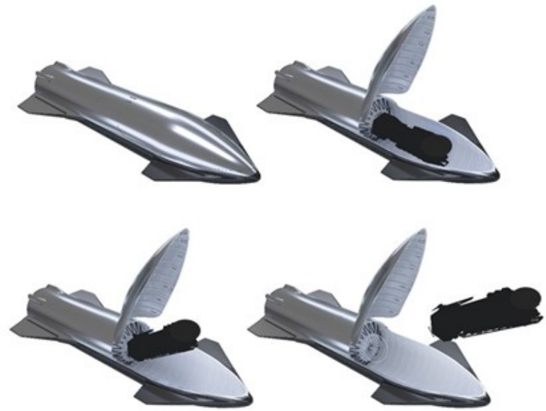
Figure 3: Starship payload deployment sequence
