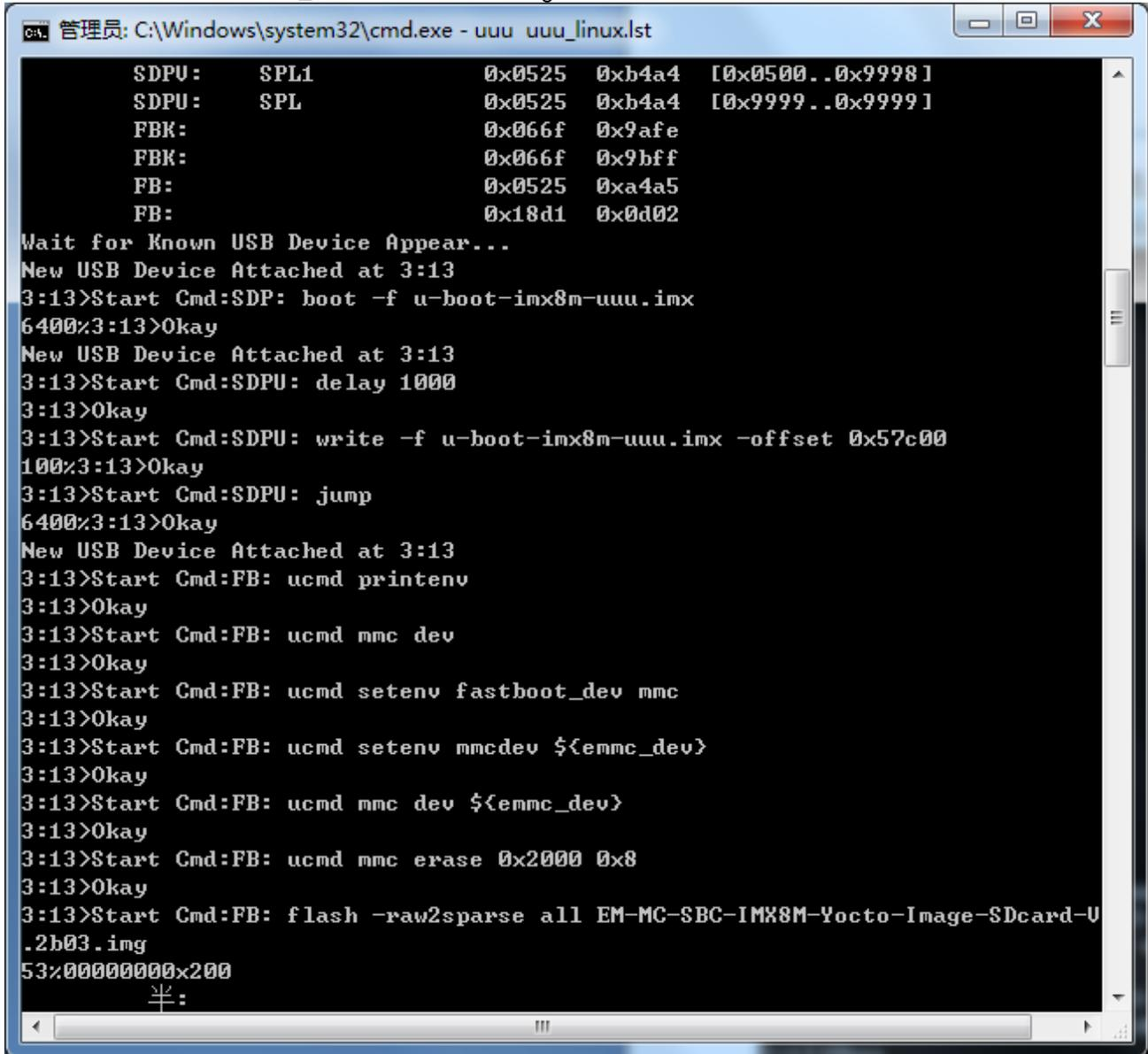
Command line will show the rate of process, while the serial terminal will print similar information until the burning finished.
