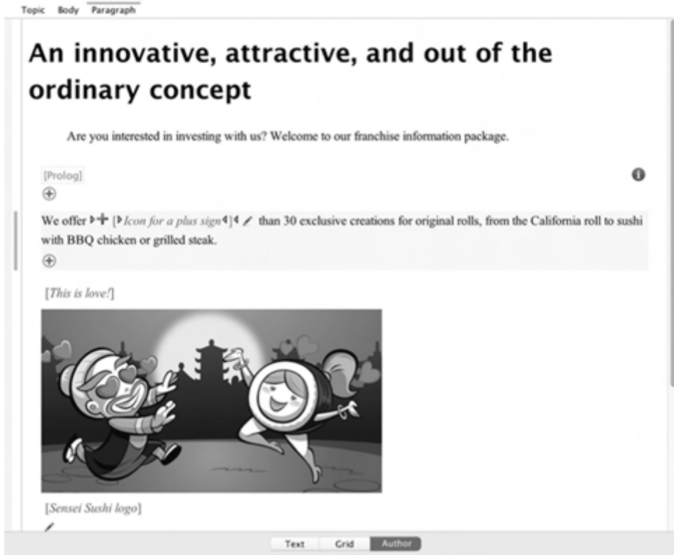
FIGURE 6.27 Preview of the XDITA topic with image and figure environments in Oxygen XML author mode. The image is in line with its containing paragraph, whereas the figure is its own block environment.
