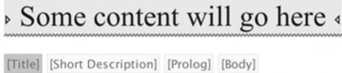
FIGURE 6.2 Validation error reported by Oxygen XML Editor. Oxygen validates the XDITA topics as the authors develop them. In this case, the “red squiggly of doom” error tells the authors that the topic is not valid and must be fixed.
