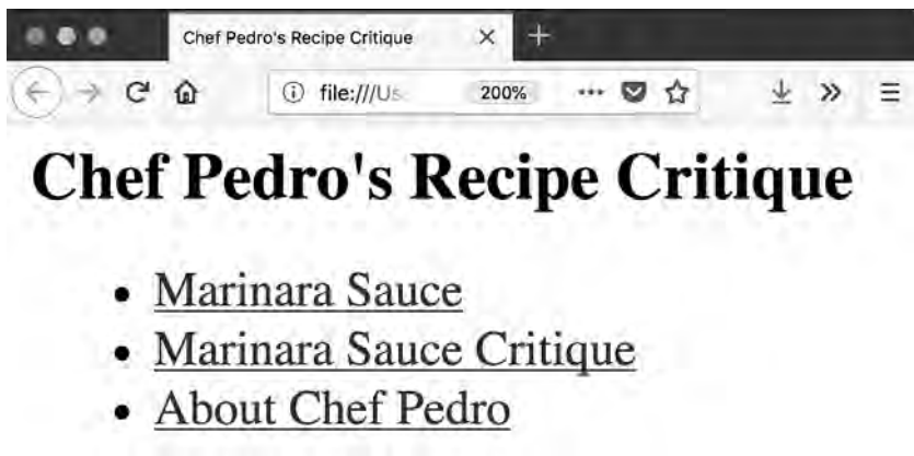
FIGURE 1.7 Navigation menu for a web transformation of Chef Pedro's recipe critique project. The DITA-OT generated the menu and took care of basic layout for this web deliverable.
