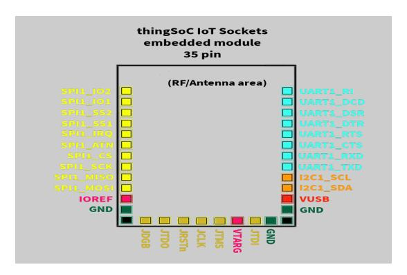
The thingSoC specification allows socket configurations from six (6) pins to thirty-five (35) pins for a single module. Multiple modules (double, triple, etc.) can be used to support a range of sizes, from small breakout boards to larger, high density input/output boards.
