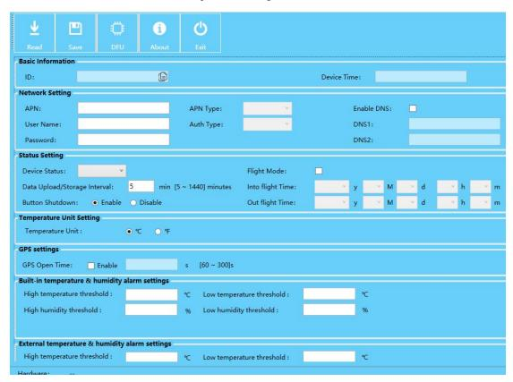
2. After the two LEDs turn on normally, click "Read" to read the machine interface parameter configuration.
