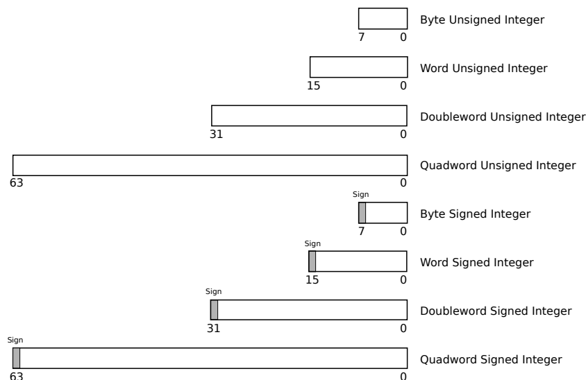
Figure 4.8.1: Fundamental Data Types
