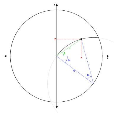
In the above diagram, R is the length of the extruder arm which is 160mm on this machine. To simplify calculations all angles will be in radians.
