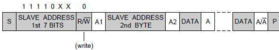
Figure 19- 14 10bit addressing, the master writes data to the slave
