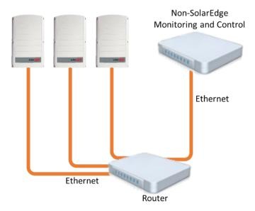
Connection to a non-SolarEdge monitoring device (with connection to the SolarEdge monitoring platform)
