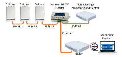
If required, use the RS485-E bus for connecting a second chain of inverters.
