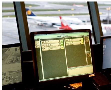
Electronic flight progress strip system at São Paulo Intl. control tower – ground control.
