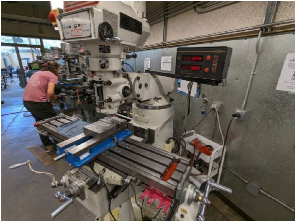
Figure 2.25: Manufacturing of go/no-go gauge on mill in Mustang '60 Machine Shop
