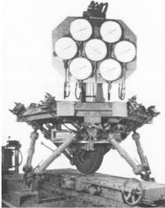
Figure 2.2: Gough's hexapod platform [2]
