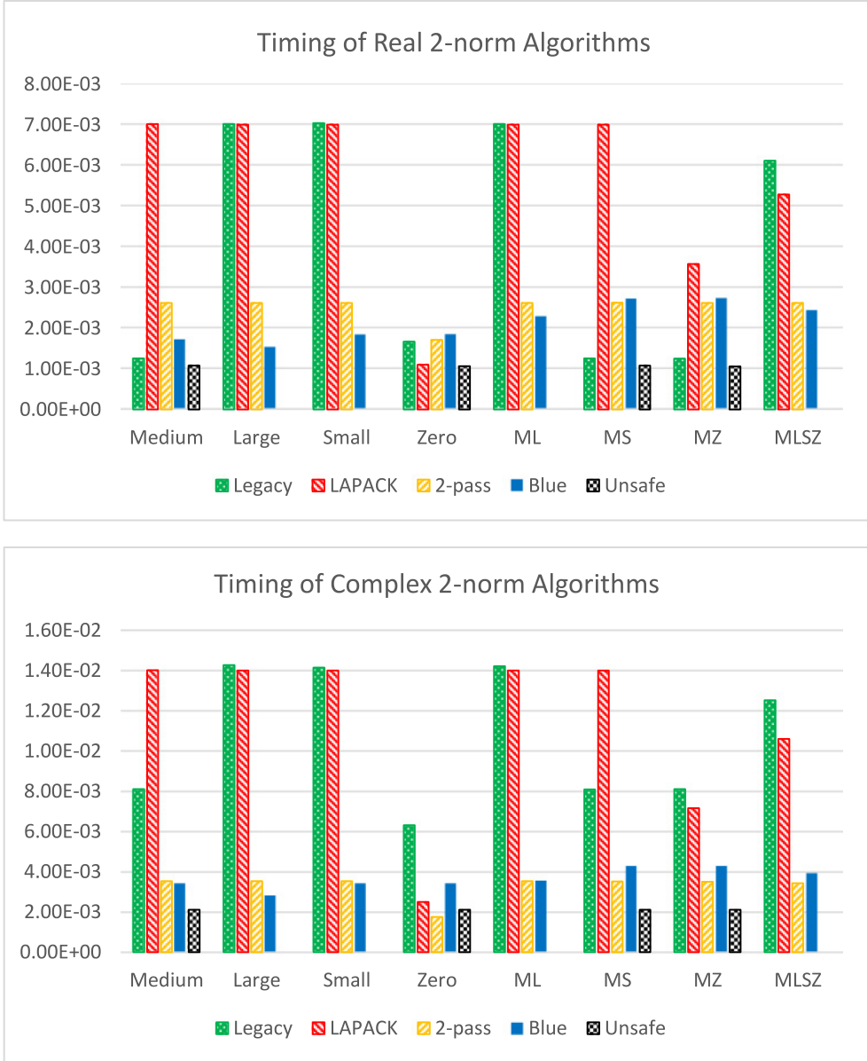
Fig. 1. Out-of-cache timing comparison of DNRM2 and DZNRM2 variants on one core of an Intel Xeon E5-2670 processor (2.6GHz, 20 MB cache), n = 1,000,000 ; time in seconds (lower is better).
