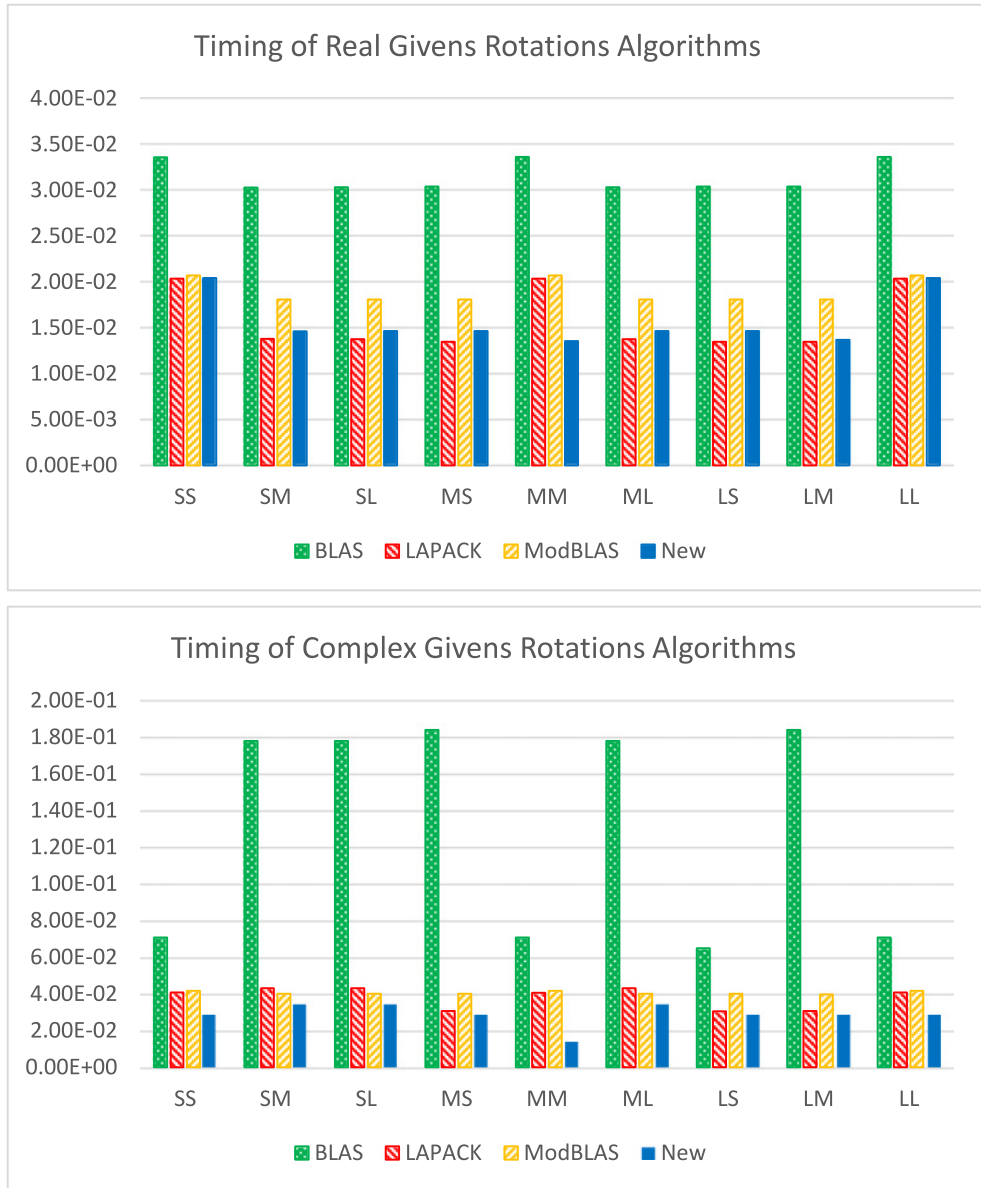
Fig. 2. Out-of-cache timing comparison of DLARGV and ZLARGV variants on one core of an Intel Xeon E5-2670 processor (2.6GHz, 20MB cache); n = 1,000,000 ; time in seconds (lower is better).
