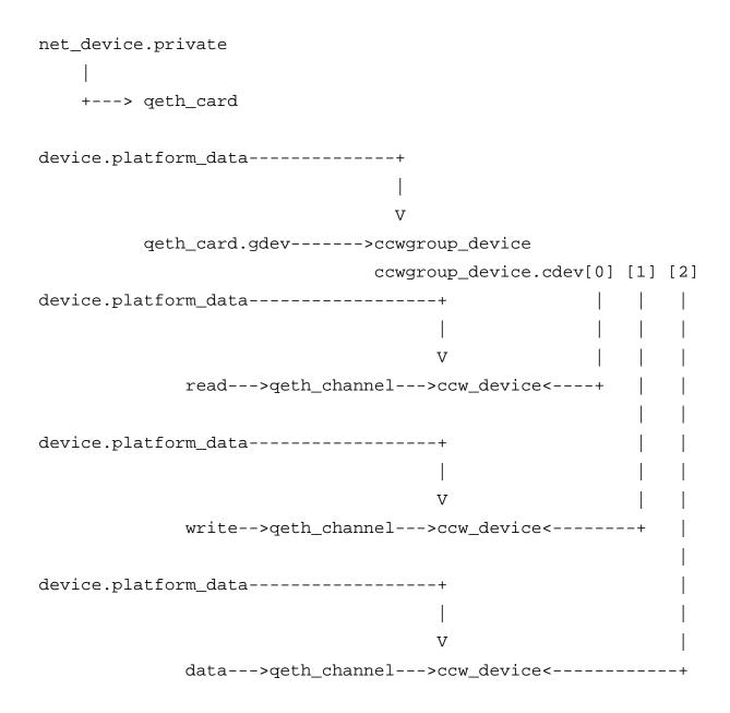
Initialization of the QETH driver is performed via net/qeth\_I2\_main.c/qeth\_I2\_set\_online. This function is identified in the CCW group driver structure.
