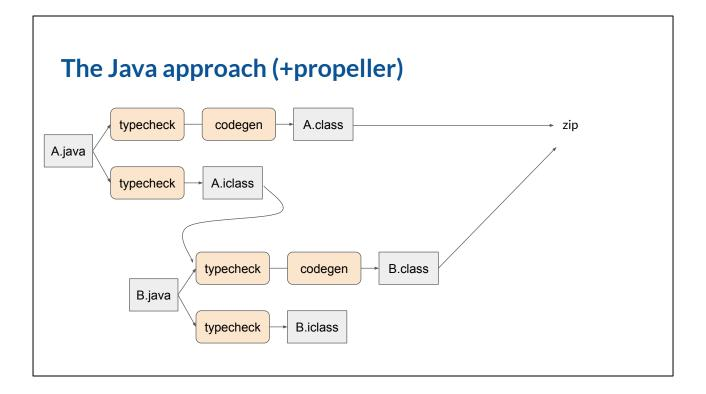
A later approach ("propeller") ran two tasks in parallel:
