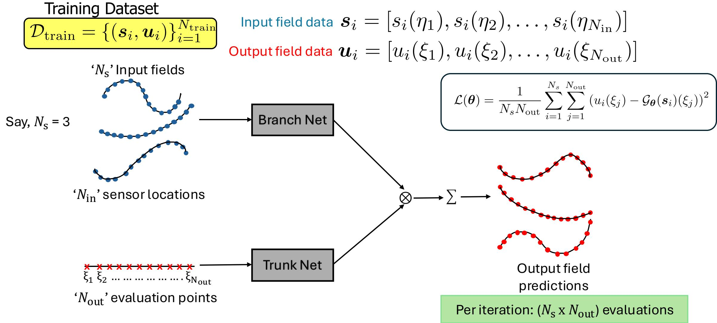
In each iteration of training for a given input field, output field is evaluated at all ' $N_{\text{out}}$ ' sensor locations.
