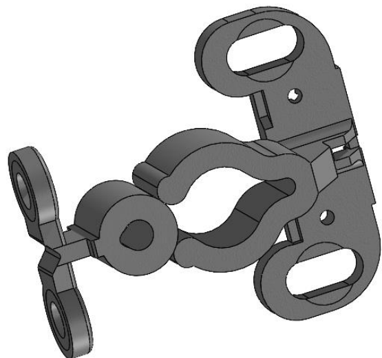
Fig 7.3: Final design of Door Catcher
