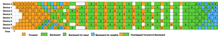
Figure 17: the DeepSeek v3 pipeline schedule (from their recent paper). Orange is the forward matmul, green is the dL/dx matmul, and blue is the dL/dW matmul. By prioritizing the backwards dL/dx multiplications, we can avoid "stranding" FLOPs.
