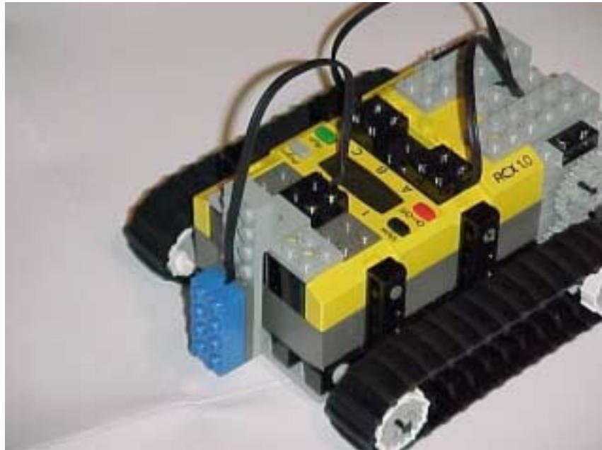
We also need the race track that comes with the RIS kit (This big piece of paper with the black track on it.) The idea now is that the robot makes sure that the light sensor stays above the track. Whenever the intensity of the light goes up, the light sensor is off the track and we need to adapt the direction. Here is a very simple program for this that only works if we travel around the track in clockwise direction.
