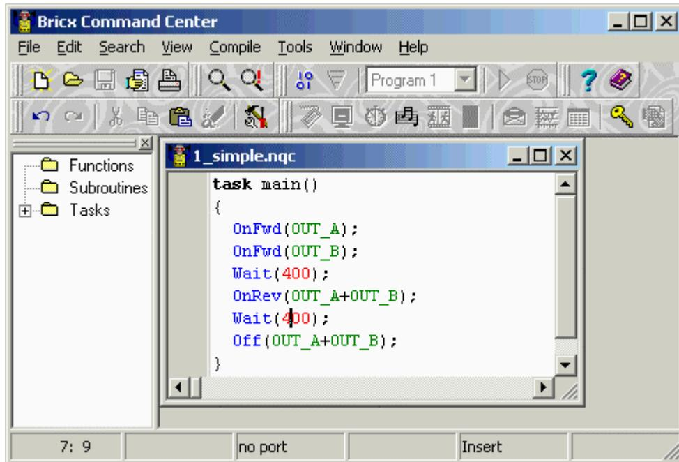
The interface looks like a standard text editor, with the usual menu's, and buttons to open and save files, print files, edit files, etc. But there are also some special menus for compiling and downloading programs to the robot and for getting information from the robot. You can ignore these for the moment.
