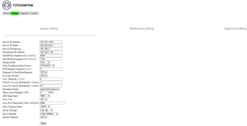
Figure 15 Web Side Lidar Setting Information
