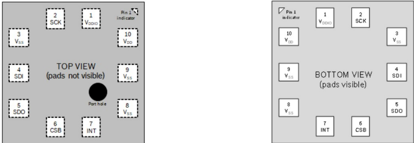
Figure 18: Pin out top and bottom view
