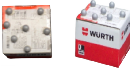
Figure 2: Exemplificative markers used to track the position and orientation of the cube with a motion capture system (e.g., OptiTrack).
