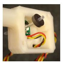
Secure the cover with two #4x3/8" screws. The slotted holes in the cover allow you to adjust the tension between the disk and the filament. You want just enough tension that the filament feeds reliably, and the disk rotates reliably.
