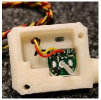
Slip the magnetic disk over the filament, and install the cover.
