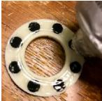
Slip the magnet wheel onto a spool support bearing that will spin reliably when the spool rotates. Make sure the wheel is aligned straight, so it spins without wobbling. Use a bit of glue to secure it to the bearing if necessary.
