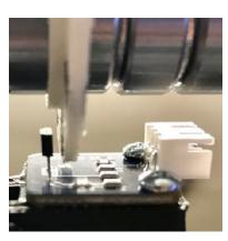
Mount the Hall sensor board in such a way that the magnets pass near the sensor as the wheel rotates. The sensor is more sensitive to one magnetic pole than the other, so you can adjust the characteristics of the output pulse by changing the orientation & distance between the sensor and the wheel.
