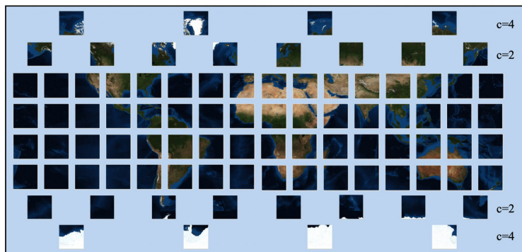
Figure 4. An example of a variable width Tile Matrix (level 2 of the GNOSIS Global Grid )
