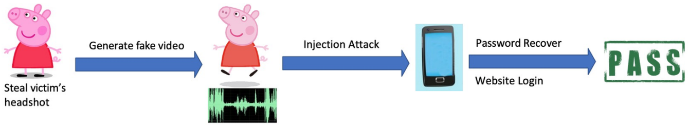
Figure 1. video injection to bypass liveness detection
