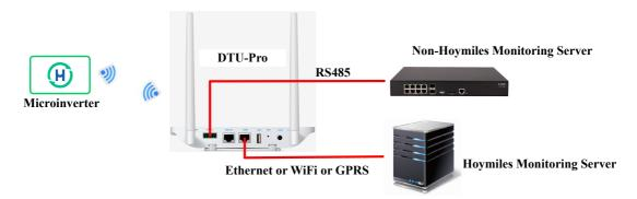
If there is more than one DTU involved in the installation, the RS485 port of DTU-Pro is connected directly to the RS485 port of third party monitoring device in turn.
