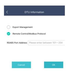
The RS485 port address needs to be set between 101~254. If there is more than one DTU in a microinverter system, the port address needs to be set up differently.
