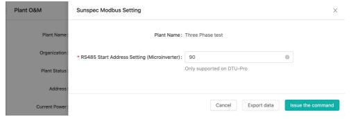
Note: RS485 addresses of all the microinverters should be within the range of 0~255
