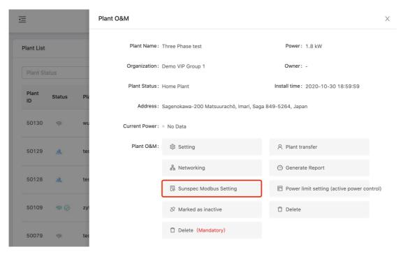
Usually there are multiple microinverters in one PV station, and all the address should be given. For convenience, after the installer completing PV station creation, only the RS485 start address need to be set for all the microinverters.
