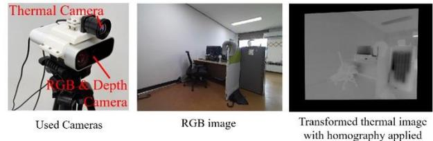
Fig. 1. Align RGB & Thermal using Homography
