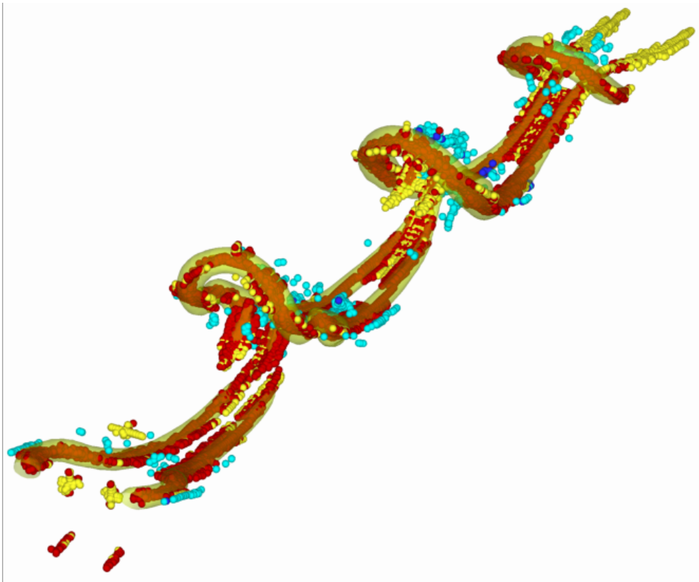
Figure 5.2: Isosurfaces of Q and extremums detected by the extrema algorithm for a 20 \times 10 \times 5 simulation instantaneous velocity field
