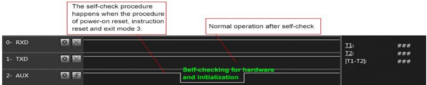
Timing Sequence Diagram of AUX when self-check
