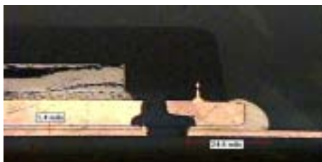
(a) 37% paste coverage, Plugged via, 1.4 mils standoff
