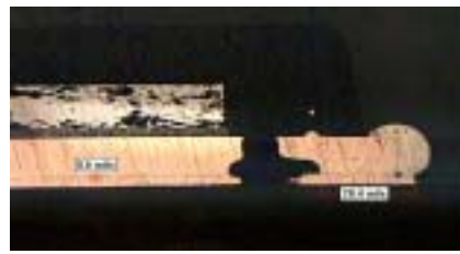
(b) 37% paste coverage, Encroached via, 0.6 mils standoff
