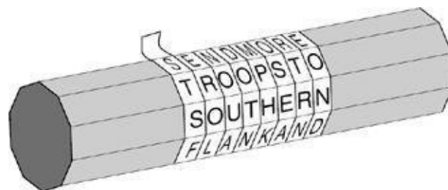
Figure 2 When it is unwound from the sender's scytale (wooden staff), the leather strip appears to carry a list of random letters; S, T, S, F,.... Only by rewinding the strip around another scytale of the correct diameter will the message reappear.
