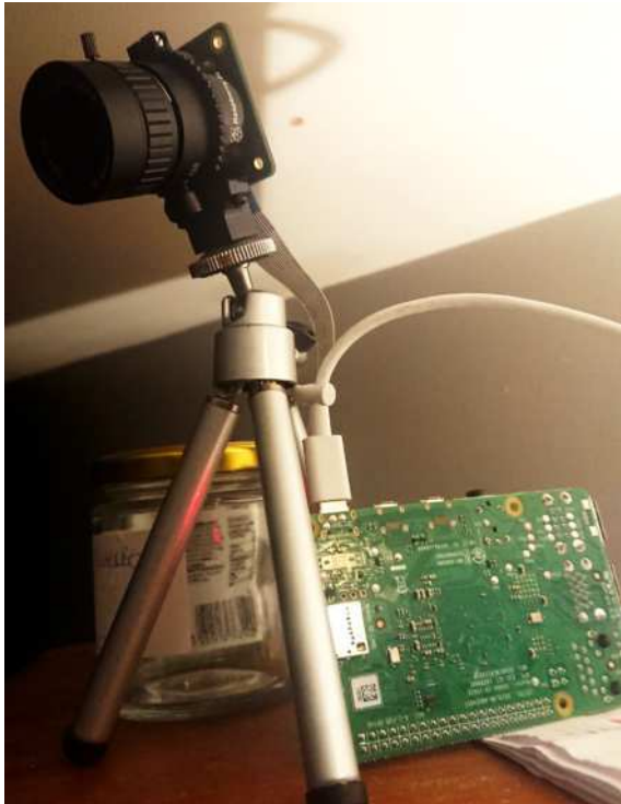
The HQ Camera has a standard tripod mount. Handy because clumsy cabling will easily topple whatever else you balance it with.
