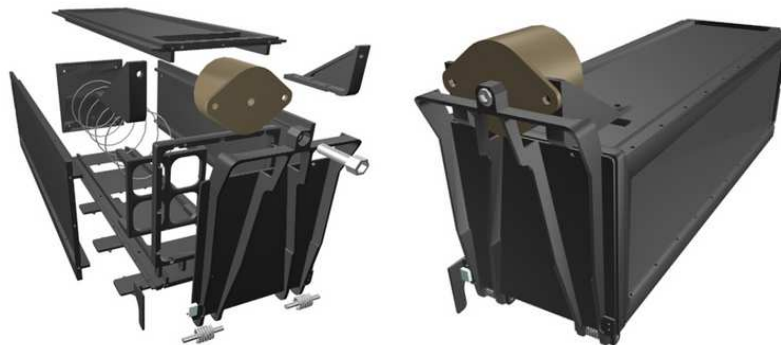
Figure 1.2: The Poly Picosatellite Orbital Deployer (P-POD) in exploded view (left) and normal view (right)
